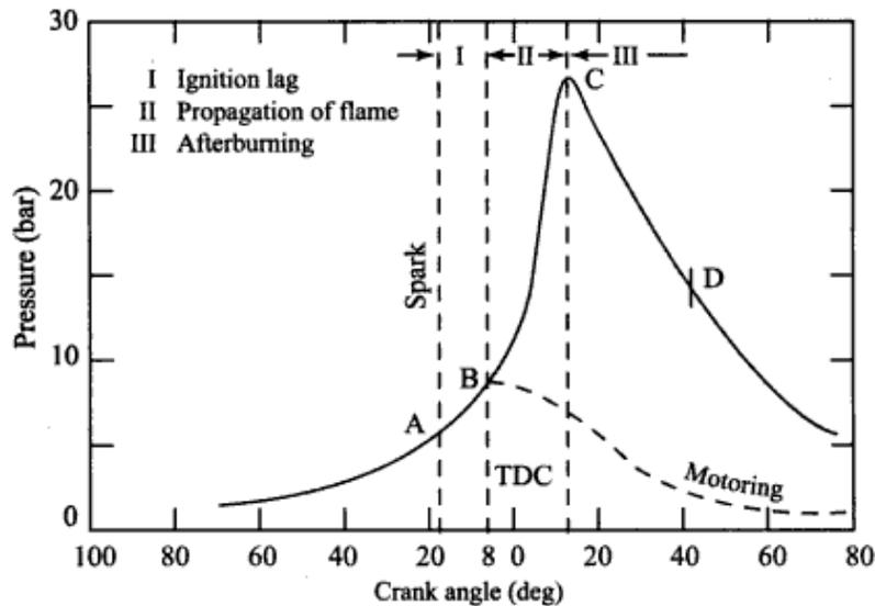
Fig. Stages of Combustion in an SI Engine
