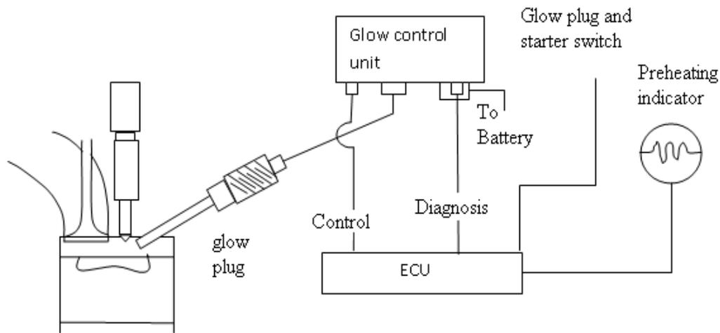
ECU Controlled Glow Plug System on D.I. Engine
