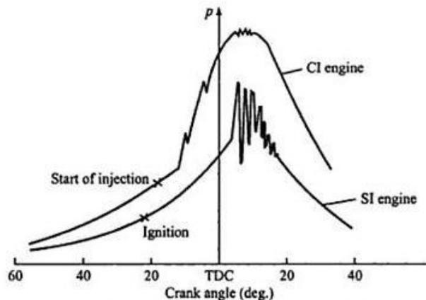
Figure Comparison of knock in SI and CI engines.
