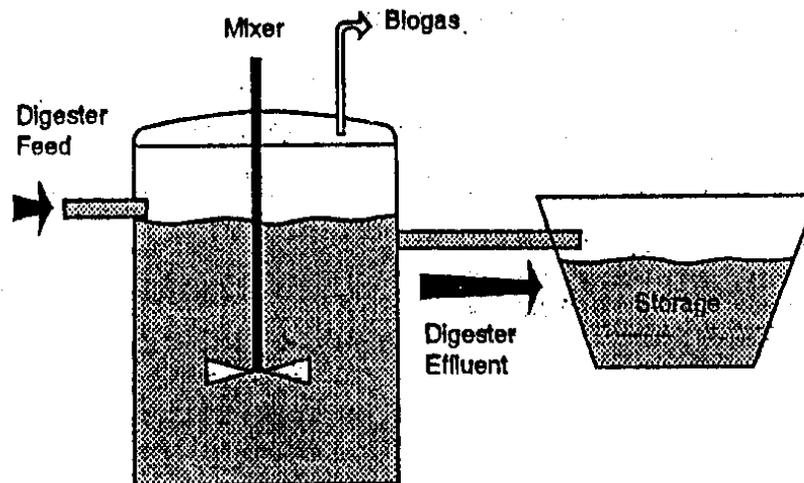
Figure shows a complete mix digester. It converts organic waste to biogas in a heated tank above or below ground. A gas mixer keeps the solids in suspension. The reactor is a circular steel or poured concrete container. During the digestion process, the manure slurry is continuously mixed to keep the solids in suspension. Biogas accumulates at the top of the digester.
