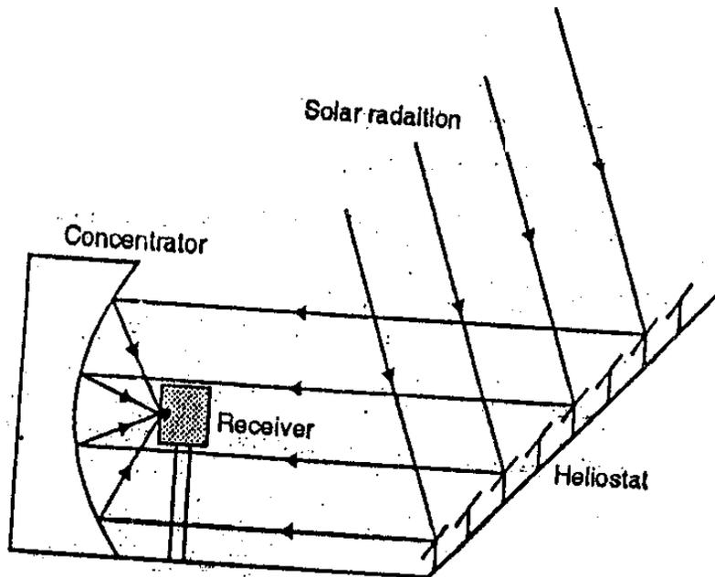
Solar furnace consists of following parts i) Bank of heliostats ii) Tower iii) Target area
