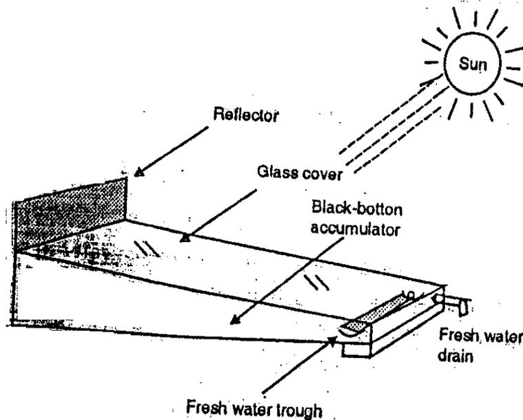
Solar distillation: Figure shows the solar distillation process. Distillation is a process that can be used for water purification. The incident solar radiation is transmitted through the glass cover and is absorbed as heat by the black surface in contact with the water to be distilled. The water is thus heated and gives up water vapor. These water vapor collected and condensed on the glass
