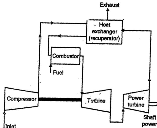
Closed cycle gas turbine Cogeneration systems: Co-generation is procedure for generating electric power and useful heat in a single installation. The useful heat may be in the form of steam, hot water, or hot air. In the cogeneration system, a mechanical work is converted into electrical energy in an electric generator and the discharged heat, which would otherwise be dispersed to the environment is utilized for useful purpose.
